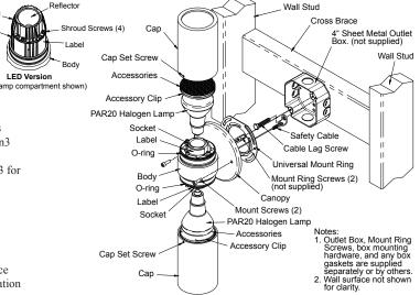
pair of fixture power leads for each LED module. Make sure that there is enough slack in the wiring so that the fixture can hang from the safety cable without stressing the wires. Note: Be sure power being supplied matches requirements on Label.
